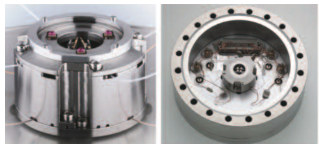
Figure 1. The ultra-compact TetraProbe STM
