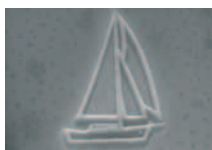
"Nano-Yacht" Bitmap Carbon deposition Orsay Physics - in house Application
