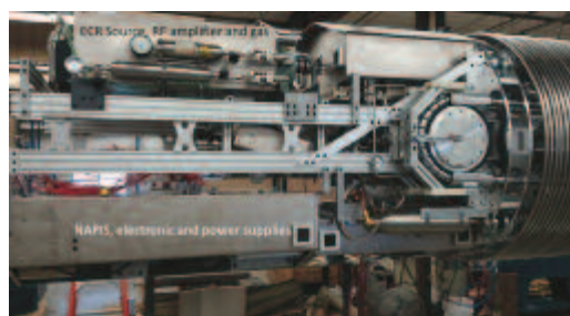
Figure 4. NAPIS and ECR ion sources installed on NEC accelerator terminal
